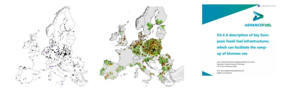
Black dots: existing coal power plant sites that are assumed suitable for construction of bio-oil units and/or biomass co-firing as stepping-stone for development of biomass market and infrastructures Purple dots: oil refineries identified as suitable for biobased feedstock (i.e., co-processing of bio-oil) Coloured areas: feedstock used to cover the demand (200 km transport limitation)
